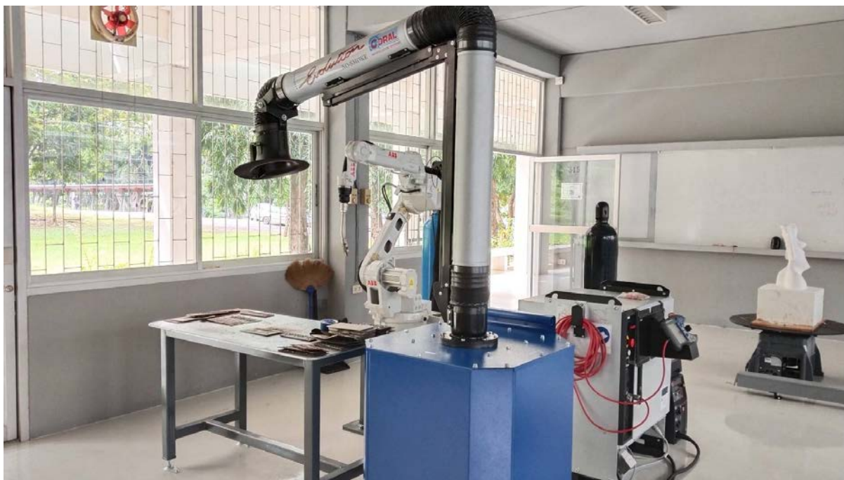
Welding robot (IRB 1520)
